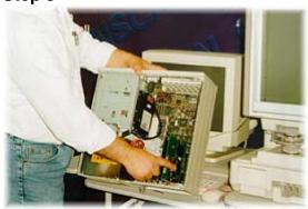
Install provided plug card in your computer, hook-up scanner cable and install software.
